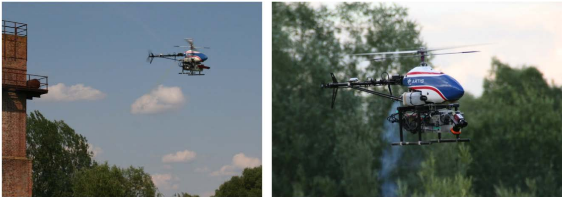
Figure 1: midiARTIS rotorcraft with onboard obstacle detection: Stereo camera (left) or a composite sensor configuration with laser scanner and camera (right).
